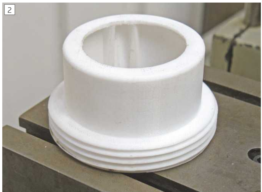
The finished protector showing detail of the thread and internal key way
