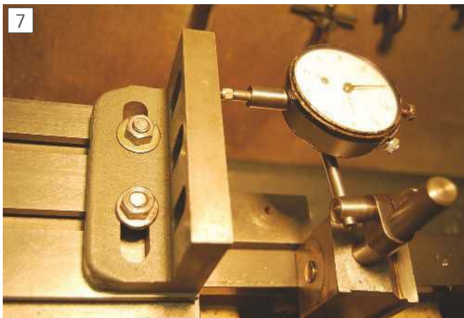
To measure saddle movement
