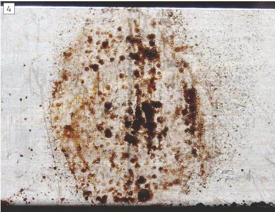
When the soap carbonises, the alloy is annealed
