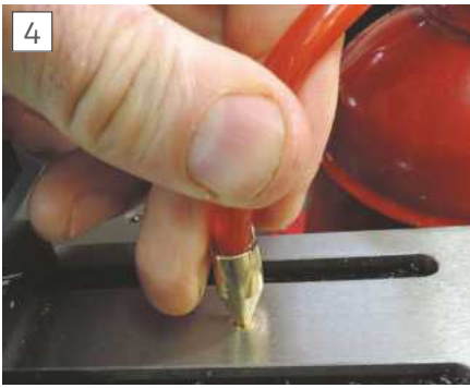
4 You can use ball oilers just by holding the nozzle of an oil can in place
