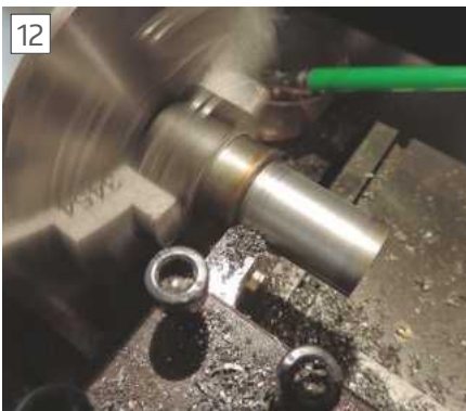
12 Cutting into a corner
