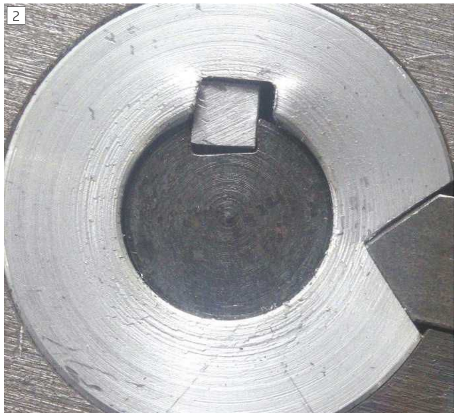
Distortion of a keyway in aluminium
