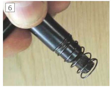
6 This spring helps stop key-in-chuck accidents
