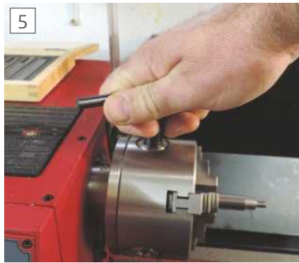
5 Always tighten a chuck single-handed
