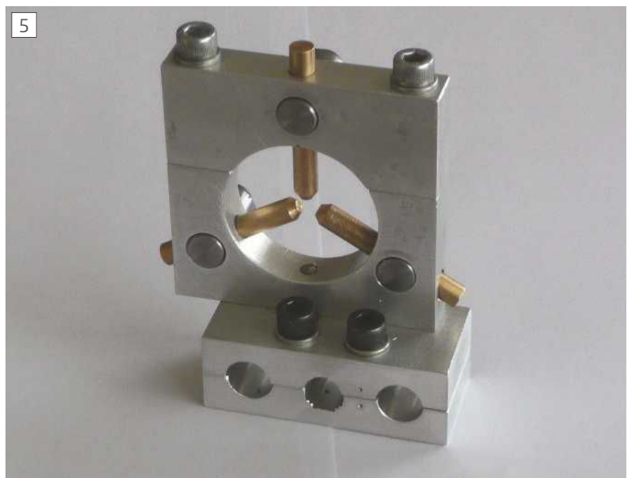
In his next article Terry Gorin describes a fixed steady for the Unimat SL 1000
