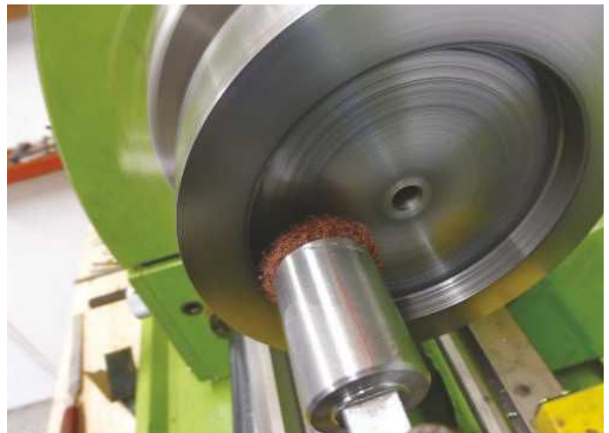
The abrasive pad is fed in under pressure.
