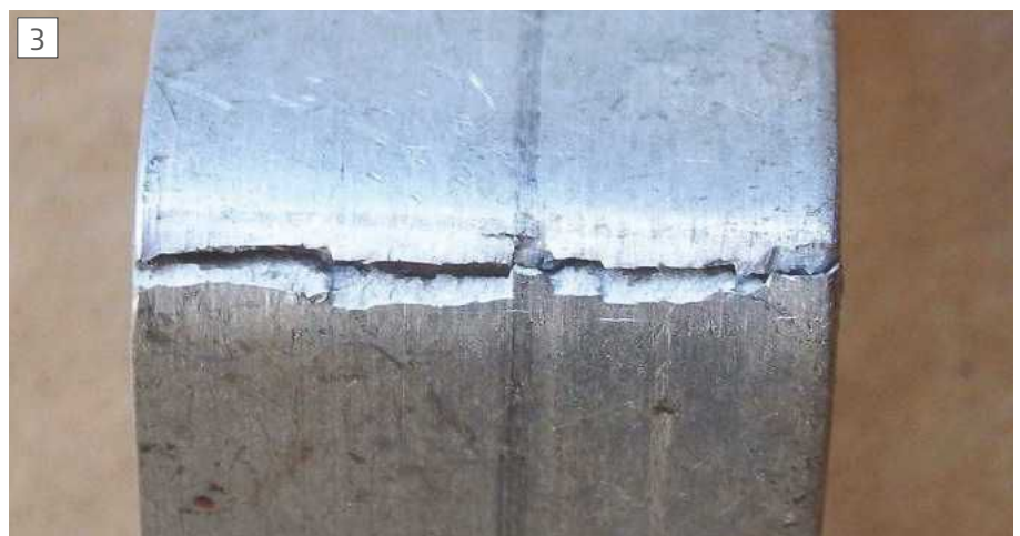
Cracking when bent
