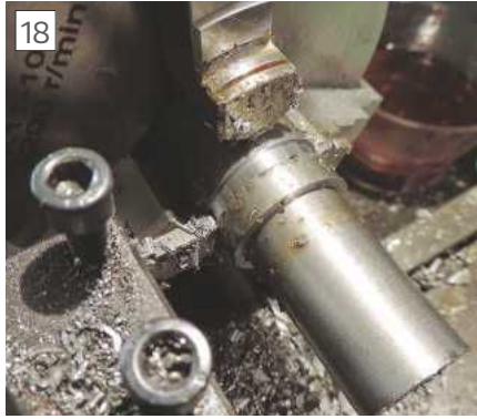
Parting off under power cross feed
