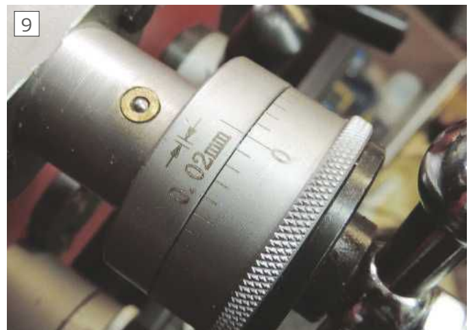
9 Use the cross slide index to keep track of the cut.
