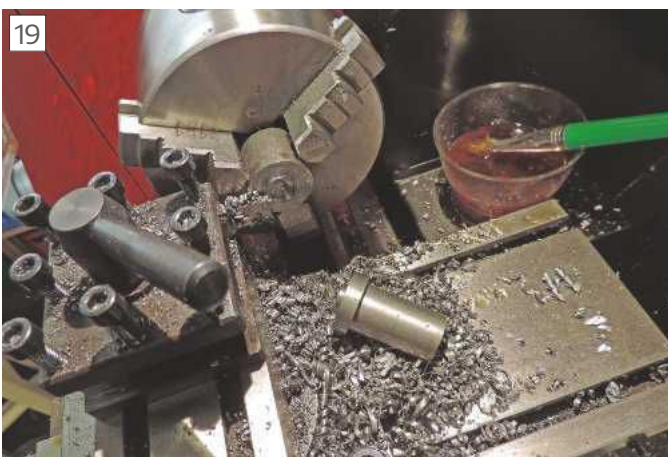
The completed part, note how parting has left a thin ring of metal around the bore.
