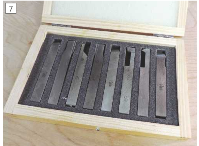
7 A typical set of pre-ground HSS tools
