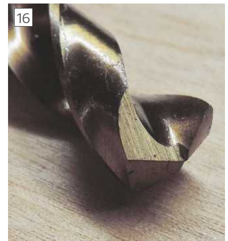
16 The tip of a split-point 5% cobalt HSS drill
