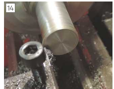
14 A cut like this is a good way to check a tool is on centre height
