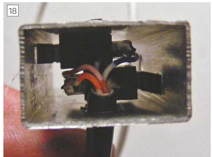
Looking inside the aluminium tube showing the micro-switches.
