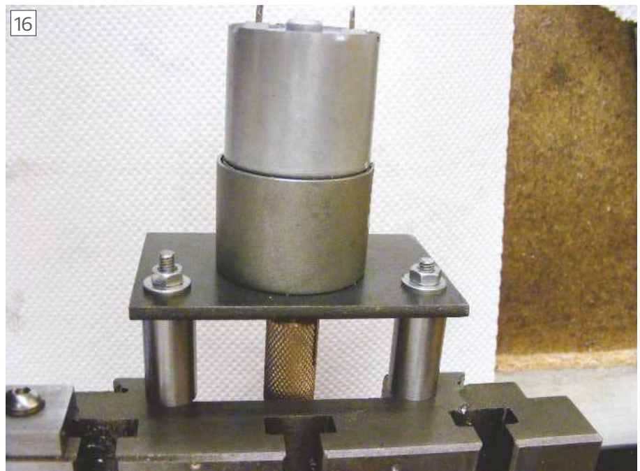
The motor plate mounted on the end of the mill table.
